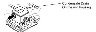
b). Vertically mounted Installation with the exhaust spigot at top. The Condensate Drain is opposite to the exhaust spigot at the base of the unit. Additional drainage may be required from the duct connected to the bottom spigot.
