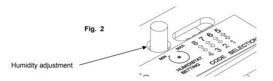
The Multivent reacts automatically to an increase in %RH above the set point value. If high humidity is detected, the fan speed increases to medium for 30 minutes. At the end of this period, if high humidity is still detected, the fan speed increases to high for 15 minutes. At the end of this period, if the humidity is low, the fan returns to its original low setting, but if still high, the fan reverts back to medium speed for 30 minutes and so on.
